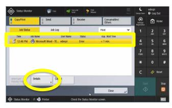
The device will indicate why the job is suspended. *I.e. No paper.*Complete the task needed to resume the job. *I.e. Place paper in the tray.*Touch **Resume**.
